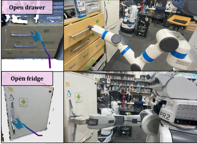
Fig. 4. Robot manipulation experiments. We visualize the generated affordances and their application to real robot manipulation tasks.
